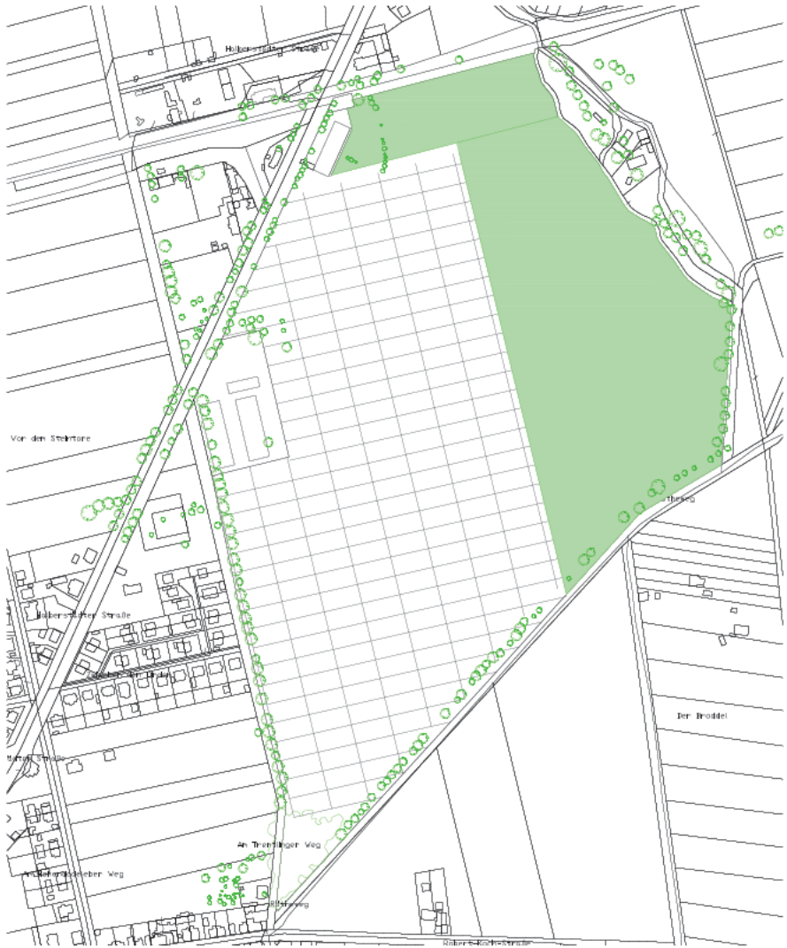
Figure 56: The generic grid of 20 m X 40 m, next to the preserved farming area in green.
