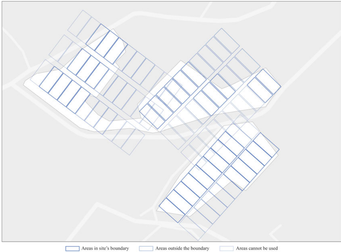
(b) The arrangement of printed blocks on the master plan is based on GHD calculations for maximum site capacity, with only the dark blue blocks deemed suitable and compliant for on-site printing using BOD2.
