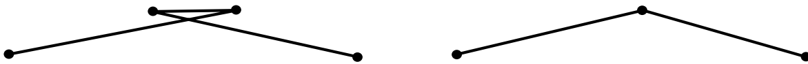
Figure 6.17: Example for removing zig-zags. The left side represents the result before and right side after the update. These zig-zags might originate from cases similar to the one displayed on the right side of Figure 6.15 due to a viewing direction which was changed just slightly in the counter-clockwise direction and minimal numerical errors during the visibility test. These can occur very easily because the viewing direction is almost parallel to the triangles.
