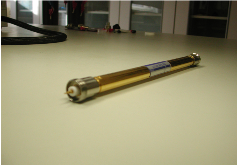
Figure 5.40: The 20 cm coaxial airline manufactured by Maury Microwave Corporation
