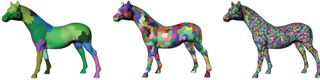
Figure 5.3: Patch hierarchies on the horse model. The first image (from left to right) shows the model with 25 patches, the second and third models have their surface subdivided in 350 and 6144 patches, respectively.
