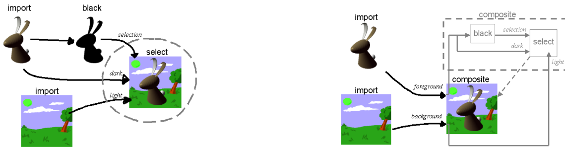
Figure 3.18: (left) Combining surface and image modifiers for a composite effect. (right) Encapsulating dataflow and remapping inputs to produce a compound modifier called composite .
