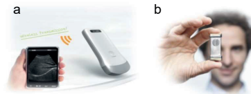
Figure 2: a) Mobile phone type ultrasound scanner, source: https://www.pinterest.com b) Tiny x-ray emitter (Tribogenics), source: https://www.wired.com
