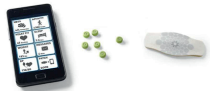
Fig. 1 - Proteus Digital Health Feedback System-The system consists of ingestible sensors embedded in tablets, a skin-worn receiver patch and a mobile device based user interface. [2]
