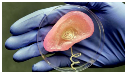
Figure 1: 3D printed ear that shows both biological and electrical part
