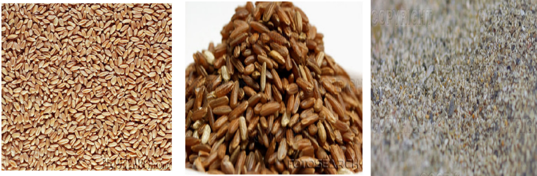
Figure 1.1: Examples of non-spherical shapes of granular materials.
