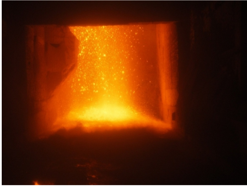
Fig.3 Clinker discharged at extremely high temperature and a falling height with 4-6m (Ch2)
