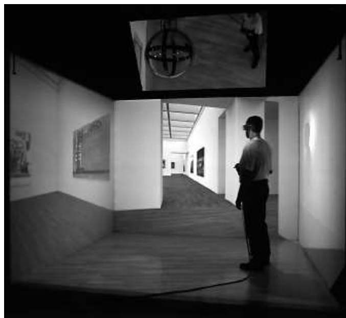
Figure E.3: CyberStage. This image shows a user exploring a museum in the CyberStage. The visible image deformations (discontinuities at the screen boundaries) are due to the physical camera position, as the displayed images are calculated with respect to the position of the user's head (which is motion-tracked). The user navigates the virtual space using a joystick-like control wand.
