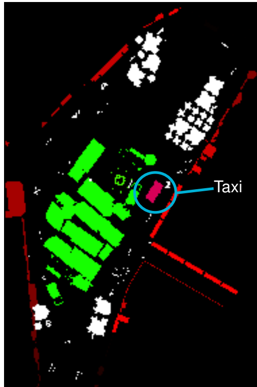
Figure 7.8: Bonn Marktplatz Hardware-Based Voxelization. This image shows the voxelization results of the state illustrated in Figure 7.9B. The shape of the moving taxi is indicated by the circle. The resolution of the voxelized data is 283x189x1. Objects which are selected for identification are rendered in different colors.
