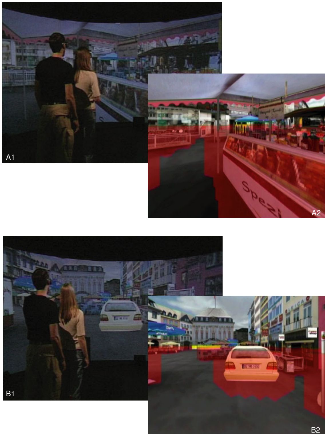
Figure 7.9: Bonn Marktplatz Application Overlaid with its Cube Space Representation. The cube space is visualized with red cubes indicating obstacles and yellow cubes indicating targets. A1 and B1 show the results in the i-Cone, A2 and B2 show the scene merged with the cube space. In A1,2, the users asked for "ice cream". The target, an ice café, is visible in the upper mid of the image. B1,2 show an dynamic object – the taxi – which moved in the way of the direct path to the distant building – the Rathaus.
