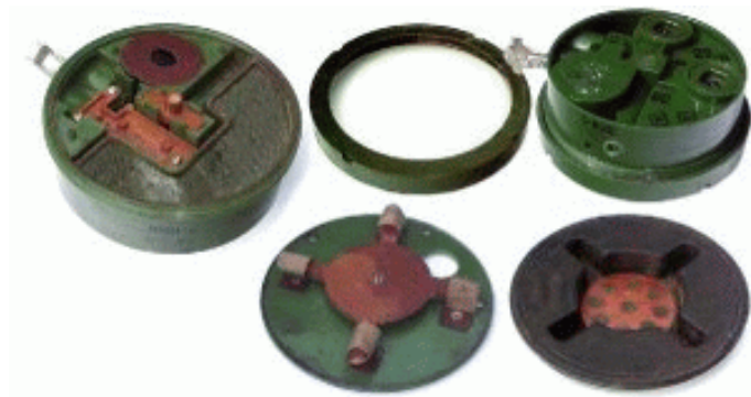
Figure B.8: Disassembled PMN-2 Anti-Personnel Mine [Smi06].
