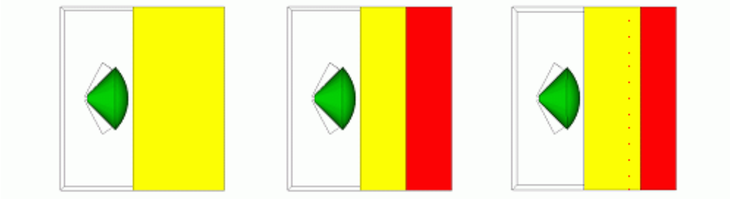
Figure 4.21: Calibration standards - match, short and different offset short.
