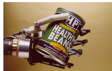
Figure 2.9: Second version of the hand of Southampton .
