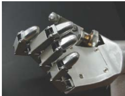
Figure 2.7: pictures of the prosthetic hand developed at the Autonomous Systems Engineering Lab of the Hokkaido University.
