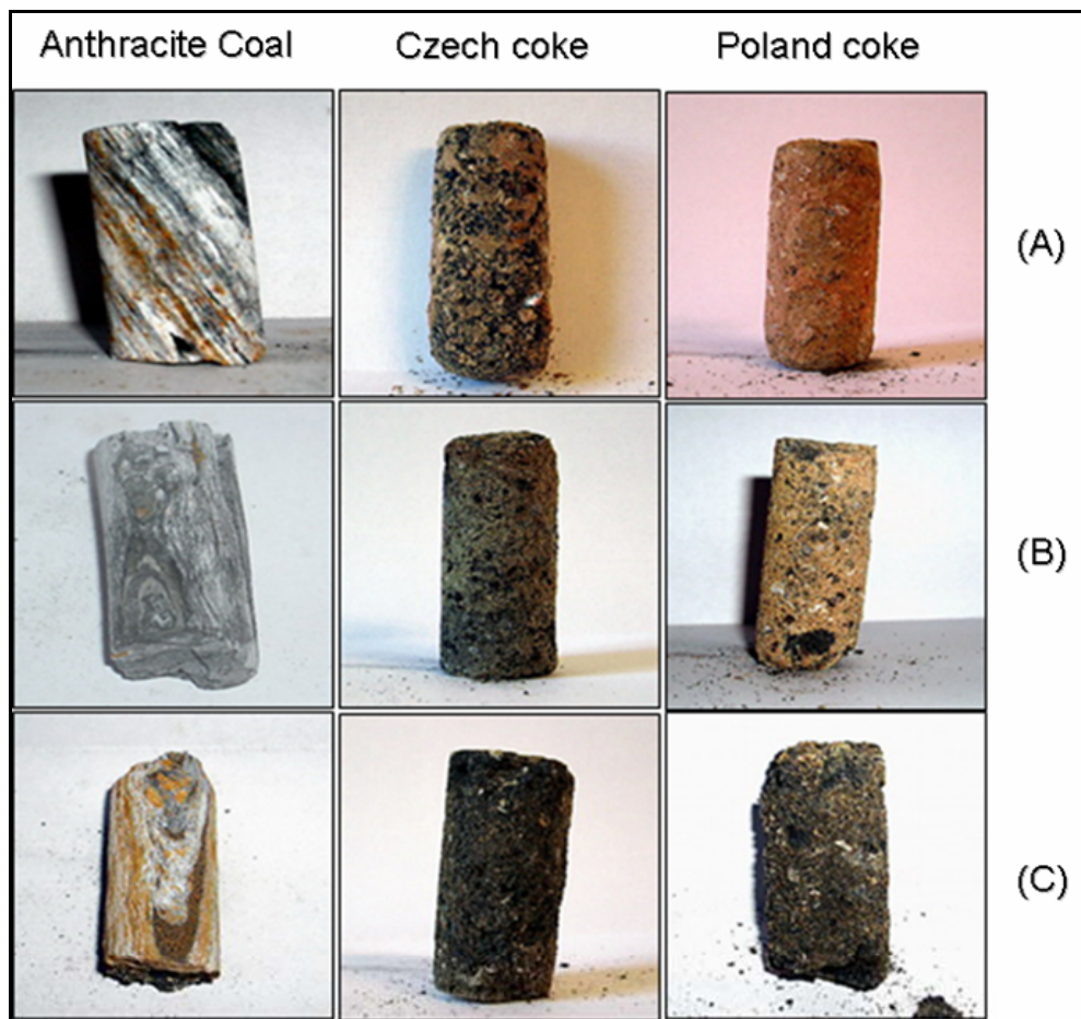
Figure 4.25: Specimen after completion of experiments. 'A' row: 900 °C, 'B' row: 1000 °C and 'C' row: 1100 °C.
