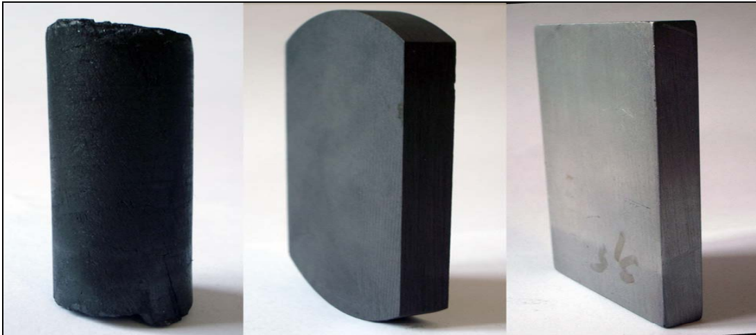
Figure 4.4: Specimens used in the experiments. Geometry (from left to right): cylindrical specimen of coke, plate of graphite, plate of aluminum
