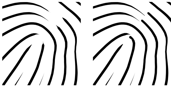
Figure 4: Computing streamline distances omni-directionally results in gaps between the tips of nearby streamlines as can be seen on the left. Using our approach these gaps are minimized resulting in the image on the right.
