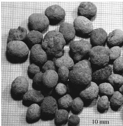
Fig. 113. Cytosap, powder-coated with lime – form and surface of granulates.
