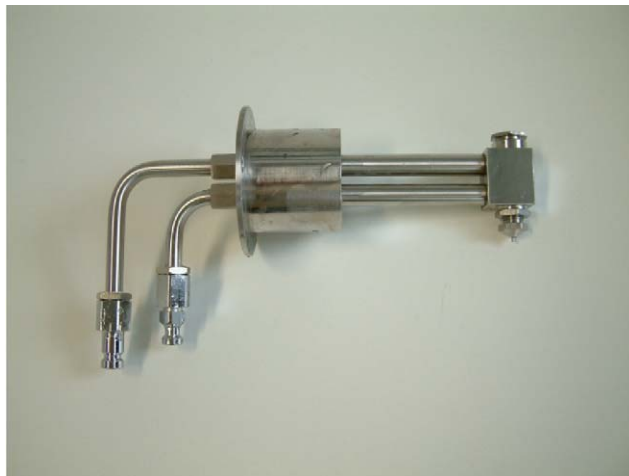
Fig. 7. Two component nozzle (Type 970/0-S04) of SCHLICK company.
