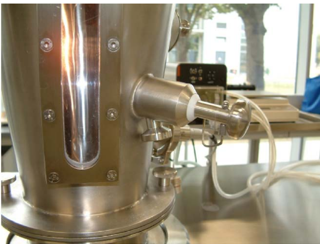
Fig. 6. Sample pipe of pilot plant.
