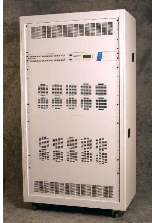
(c) Magnetlager Controller
