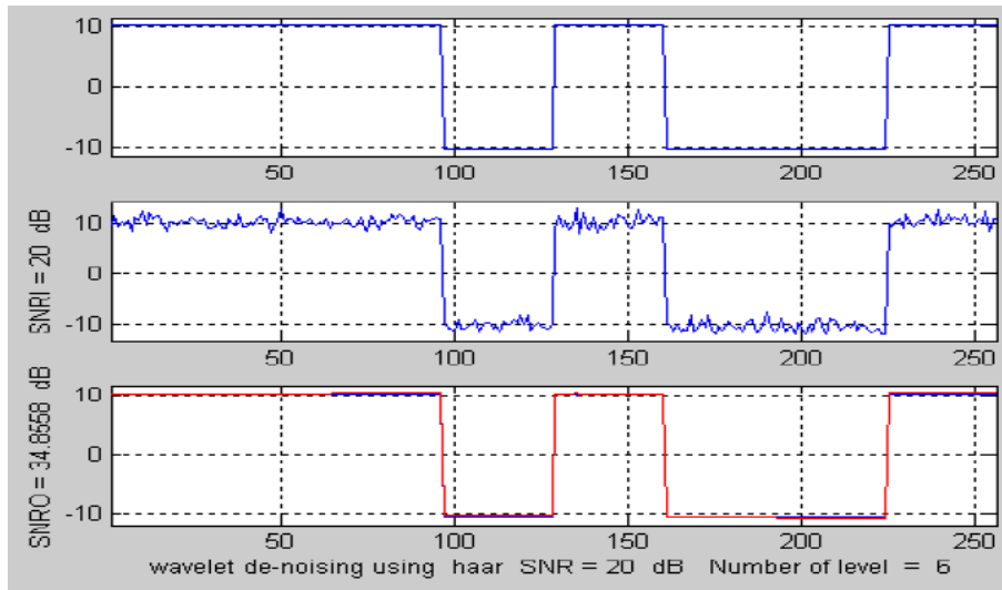
Figure 3.19: Denoising of the PN code using Harr wavelet (SNRI = 20 dB and SNRO = 34.86 dB).
