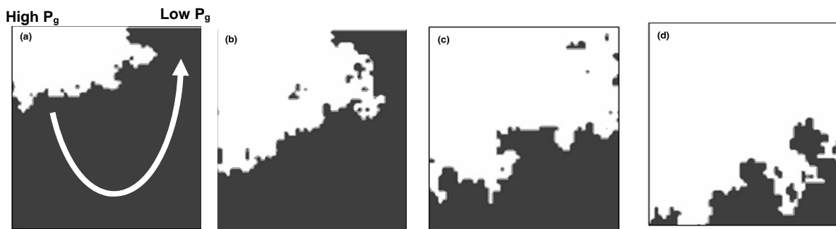
Figure 1.34: Phase distributions at high gas flow rate for saturation S = 80 \% , 60 \% , 40 \% and 20 \% (Yiotis, et al., 2001 [37]).
