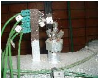
Figure 5-3. Measuring device with five thermocouples
