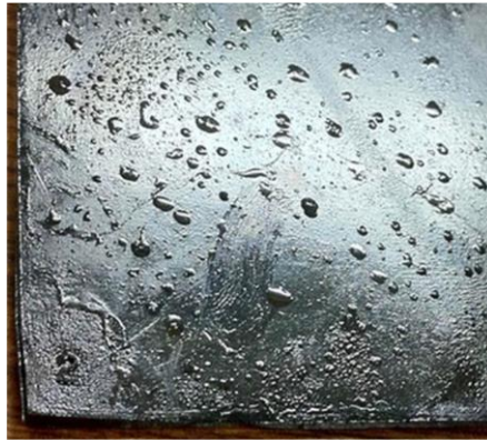
Figure 26: Bleed-out of soybean oil from cured tensile pad molded from EPDM, photo reproduced with permission from ref [151]
