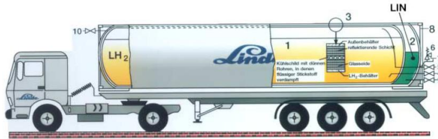
Figure 3.18 Schema of an LH 2 tank truck [Linde AG]
