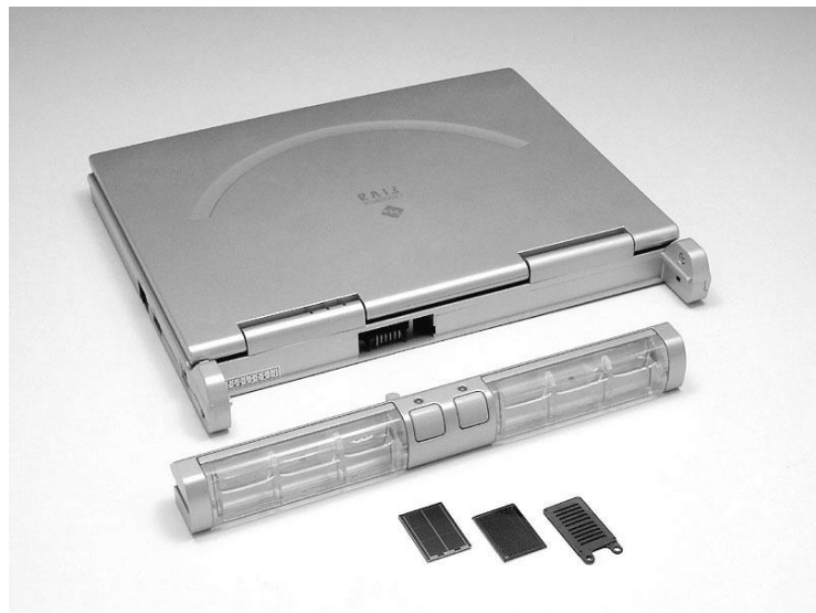
Figure 1-1 Fuel cell system for Laptop developed by Casio Corp. (Japan). System consists of hydrogen fuel cell (PEMFC) and integrated micro reformer fed with methanol-water solutions.
