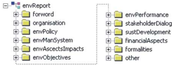
Fig. 1: Proposal of a harmonised DTD for environmental reporting on top level (Lenz/Isenmann/Marx-Gómez/Krüger/Arndt 2002, 422)
