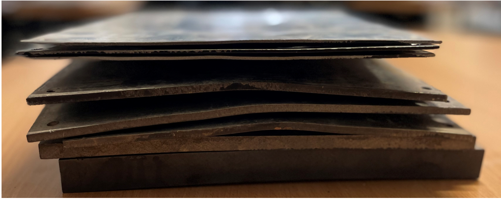
Figure 1.6: Typical distortion in quenching of hot metal plates
