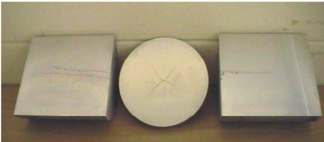
Figure 1.7: Typical hot tears which occur during pseudo steady state phase Suyitno et al. (2004)
