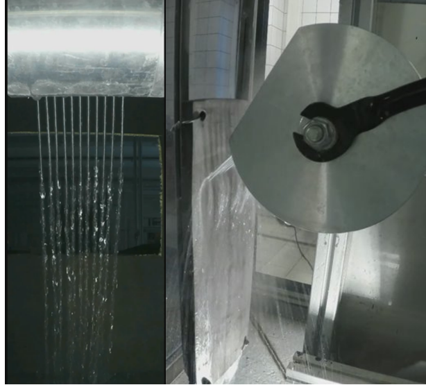
Figure 2.4: Left) Water Jet Mold used for cooling with 11 orifices, Right) Photographic visualization of quench side
