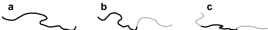
Figure 2.1: Schematic drawings of (a) a homopolymer; (b) an AB di- block copolymer; and (c) an ABA tri- block copolymer. The lighter and darker colors indicate different species of monomers A and B, respectively.
