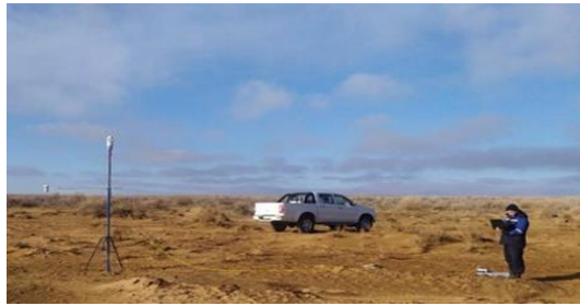
Figure 5: Measuring solar energy at a height of 2 meters and weather conditions at a height of 3 meters.
