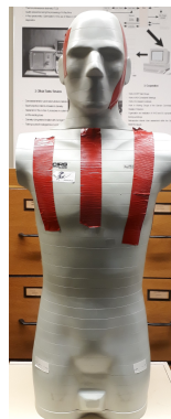
Figure 4.2: CIRS 701 Adult male phantom (Cirs Inc. USA). This phantom was designed to simulate the anatomy of the patient and for rendering more reliable and accurate CT dose data. (The phantom was provided by the Bundesamt für Strahlenschutz, Munich, Germany.)
